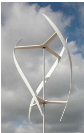
Varying scales and types of wind turbines. Left: a 6kW VAWT Right: a small 500W HAWT. Source: XCO 2
