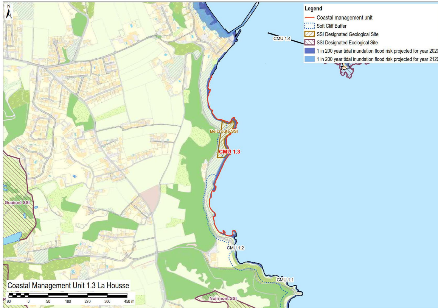
Figure 4-8: Coastal Flooding and Erosion risk at CMU1.3 (La Housse)
