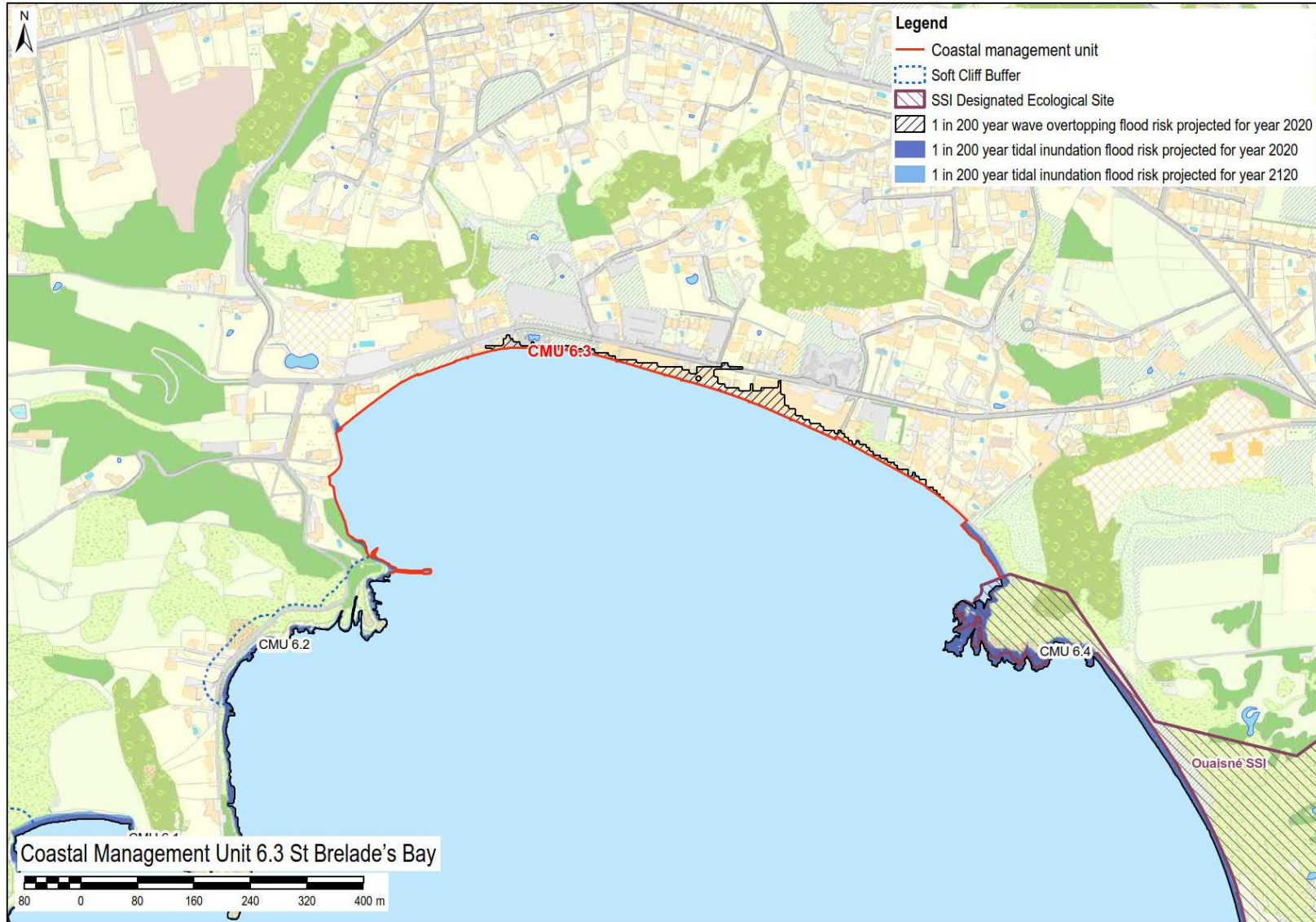
Figure 9-7: Coastal Flooding and Erosion risk at CMU 6.3 (St Brelade's Bay)
