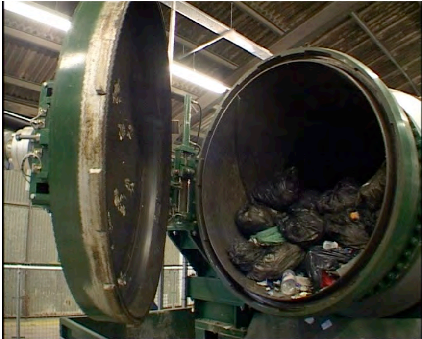
Autoclave with black-bag garbage ready for treatment (S. Wales Plant, 2001)
