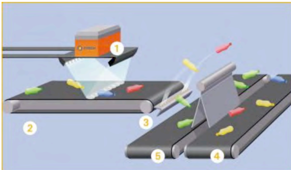
1. Scanner, 2. conveyor belt with input material, 3. air jets, 4. second transport system with ejected material and 5. residual fraction
