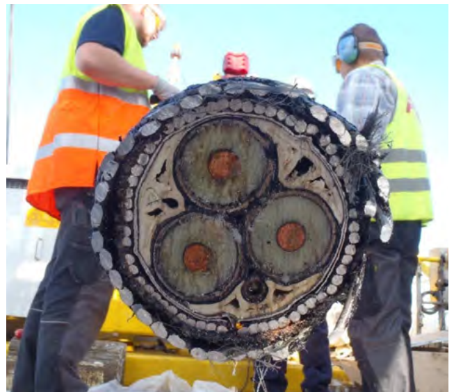
Cross-section through a submarine power cable.
