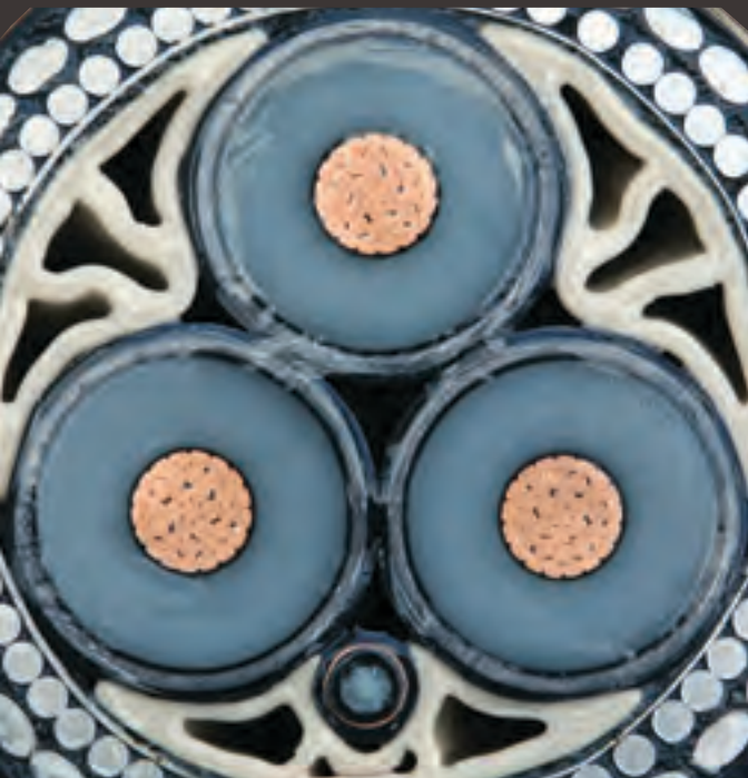
Inside Normandie 2 showing fibre optic cable laid alongside power lines.
