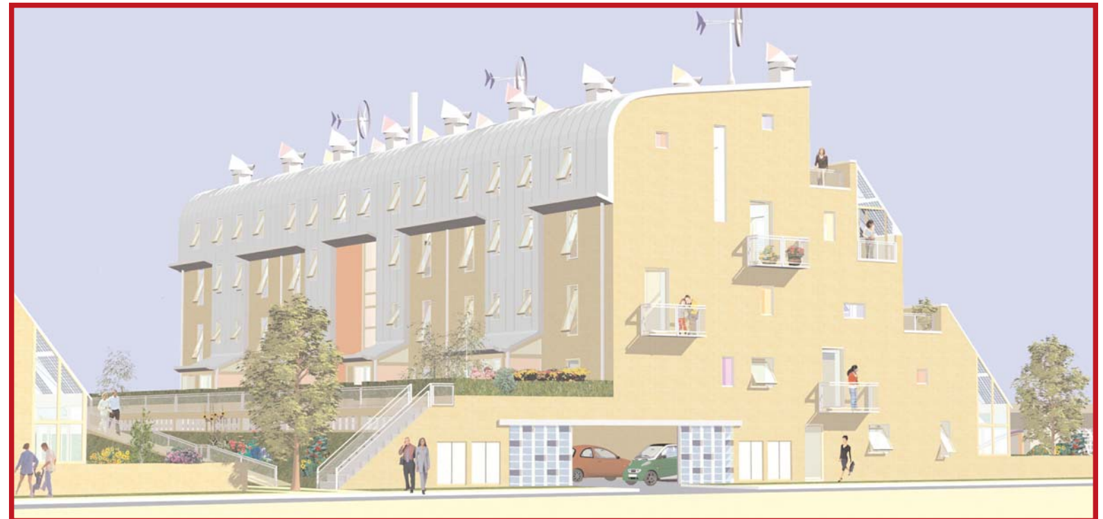
Above: Showing conservatories on South side, with building integrated PVs and some opening lights.
