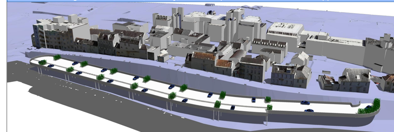
CONCEPT D: Single Deck Car Park (two-way) 90 new spaces Approx Cost: £4m
