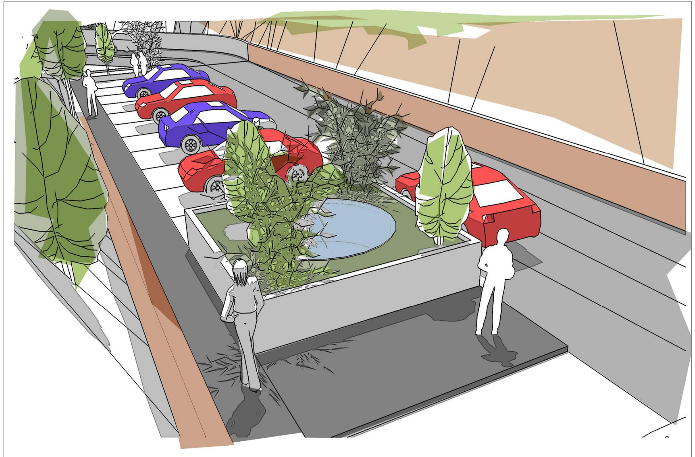
Artist's impression of planter concept incorporating light well to ensure good level of natural light to ground floor
